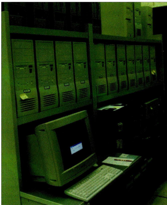
Prototype of the COMPASS computing farm. The PCs are mostly dual Pentium II 300 MHz running Windows NT 4.0 SP3. The data servers are DEC1200 and SUN 450 machines.
