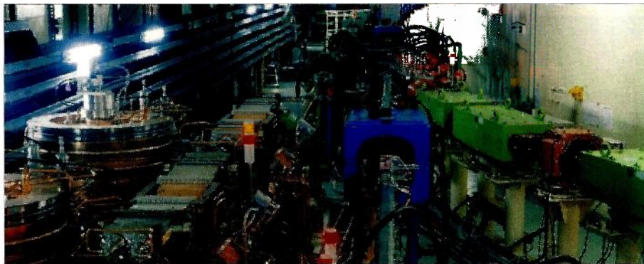
The Japanese KEKB electron-positron collider. This picture shows the injection point of the electron beam. From the right, 8 GeV electrons arrive through the beamline with light-green dipole and orange quadrupole magnets, and enter the high-energy ring with blue quadrupole magnets. A couple of ARES radiofrequency accelerating cavities for the low-energy 3.5 GeV positron ring are also visible. KEKB is in the 3 km tunnel, which formerly housed the TRISTAN electron-positron collider.
