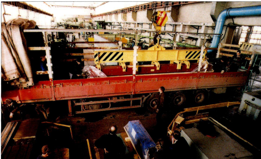
Loading a 6 m dipole magnet at Novosibirsk for the 6000 km journey to CERN. These magnets will equip the two transfer lines to feed the LHC collider with protons from the SPS proton synchrotron.
